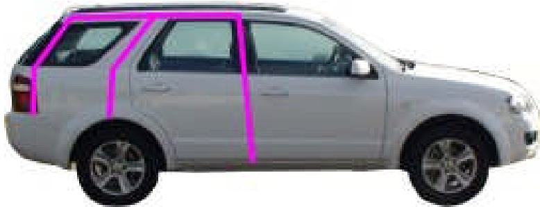
Figure LK20 Typical example of an internal ROPS fitted to a station wagon providing protection for both front and rear passengers.
